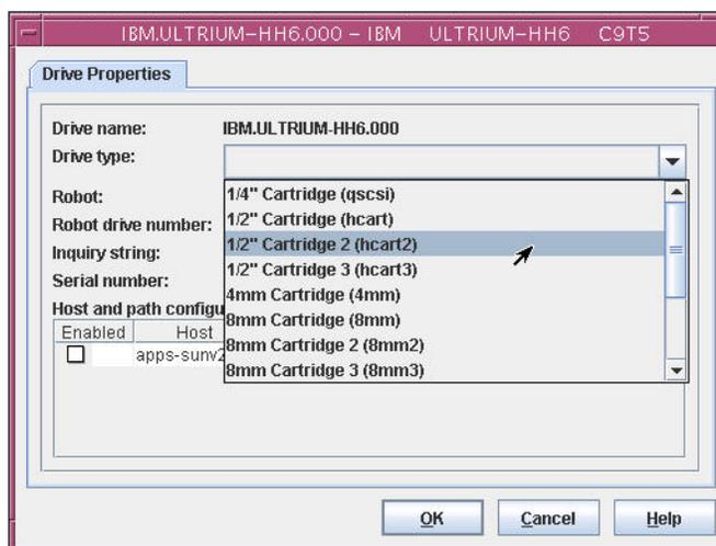
The example here is the setting for a NEO 2000e with IBM LTO-6 TD (full-height) tape drives. You must select **1/2" Cartridge 2 (hcart2)**.
