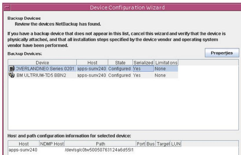
Example of a NEO 2000e and a NEO 200s with IBM LTO-6 fibre tape drives discovered:
