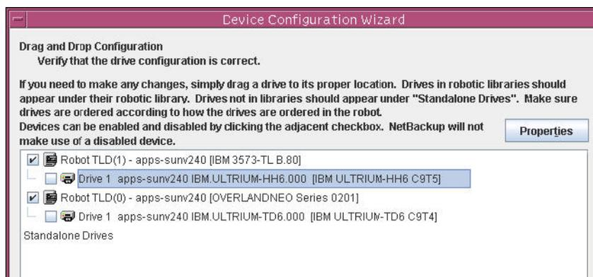
The example here is the setting for a NEO 200s with IBM LTO-6 HH (half-height) tape drives. You must select **1/2" Cartridge 2 (hcart2)**.
