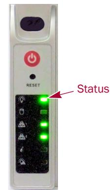
Once initialization is complete, the system automatically reboots and the Status LED displays a solid green color.
