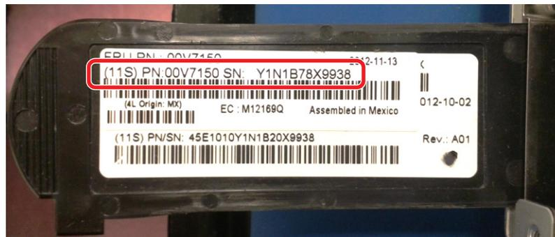
Figure 4: NEO 200s/400s Service Tag on Pull-out Tab
