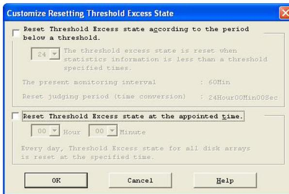
**Figure 3-9: Customize Resetting Threshold Excess State**
