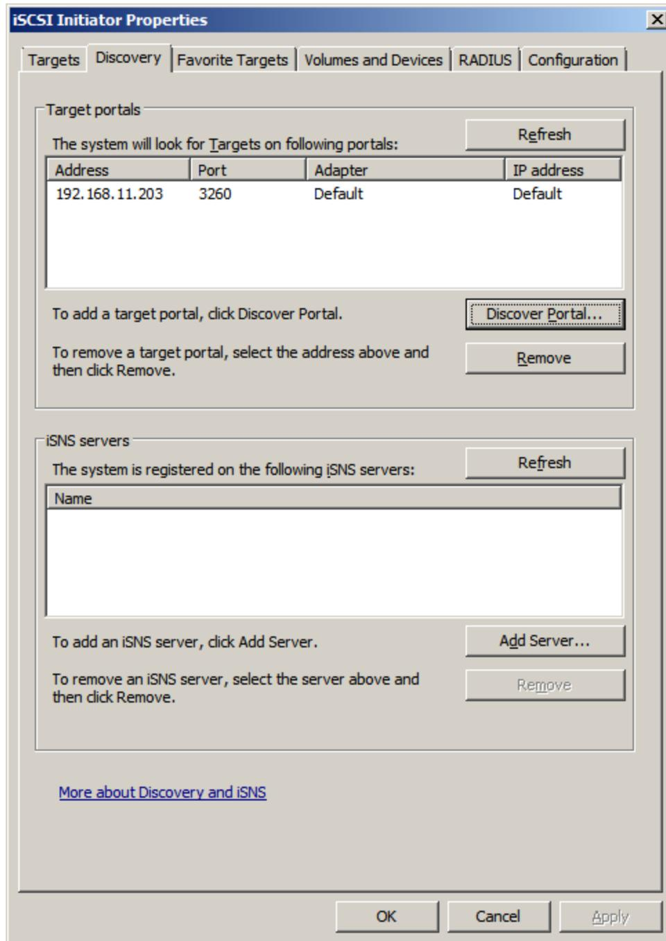
**Figure 3-46: IP Address and Port Confirmation**
