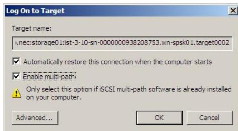
Figure 3-38: Target Options Checked
