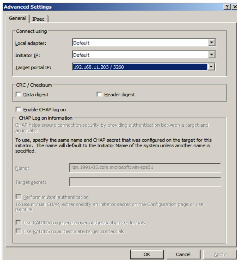
Figure 3-50: Target Portal IP
