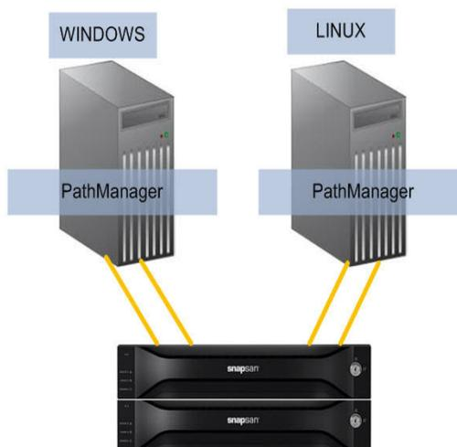
Figure 1-3: Multiple-server Configuration
