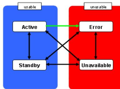
Figure 5-4: Transition of path status on failover
