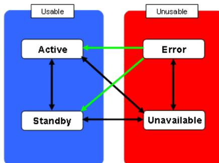
Figure 5-9: Failback By Recovery Check
