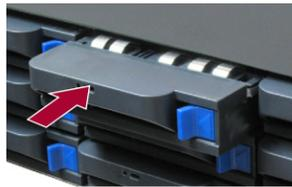
**IMPORTANT:** To maintain proper airflow and cooling, a drive assembly or a blank drive carrier must be installed in every slot. No empty slots are allowed.
