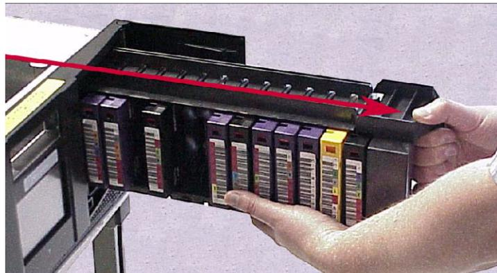
Do NOT angle the magazine up, down, left, or right, and do NOT twist or tilt it.
