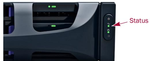
Once initialization is complete, the system automatically reboots and the Status LED displays a solid green color.
