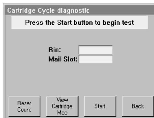
**Figure 5-26: Starting the Cartridge Cycle Diagnostic**
