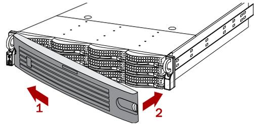
Figure 14. Attaching the Bezel
