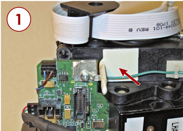
Figure 17. Secure Plastic-Coated Clamp to Shuttle
