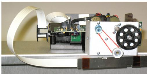
Figure 3. Set the Shuttle Aside; PCB Up
